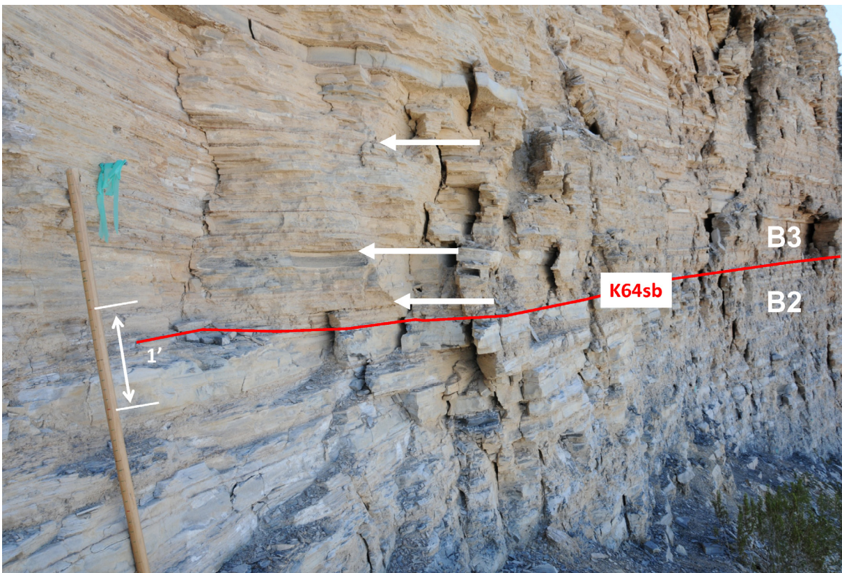
Figure 15. Boundary between sub-facies B2 and B3 at approximately 48 ft on the measured section. At this boundary, a slight color change occurs, which is associated with the onset of abundant 0.5–4.0 inch thick bentonite beds (white arrows). This boundary is interpreted as the K64sb.
