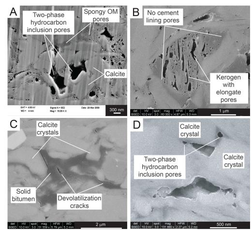
crograph of mineral pore where part of pore filled with solid bitumen or pyrobitumen containing bubbles that we interpret as having formed by two-phase hydrocarbon inclusion. Pine Island Shale Member of Lower Cretaceous Pearsall Formation, Atascosa County, Texas, Humble Pruitt No. 1, 9700 ft, measured Ro = 0.78%.
