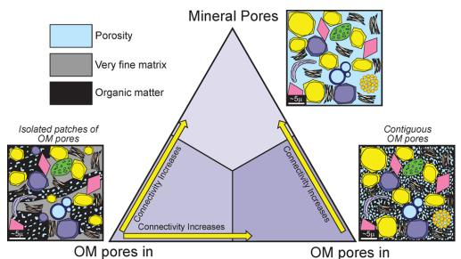
Figure 7. Ternary diagram showing end members (with schematic representations) of mudrock pore networks. Pore network can be combination of mineral pores, OM pores in depositional organic matter, and OM pores in migrated organic matter. We suggest that, as proportions of OM pores in migrated organic matter and mineral pores increase, connectibility increases, resulting in better permeability pathways.
