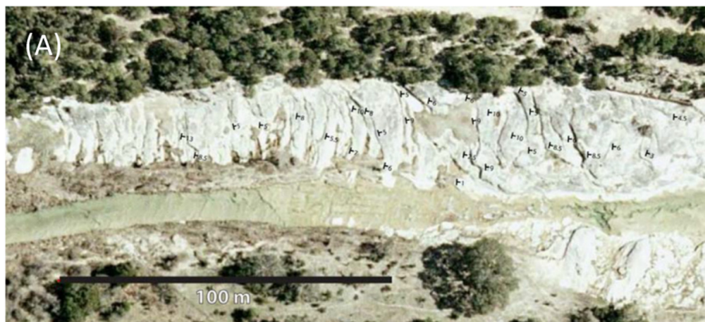
Figure 4. Map view snapshots from the outcrop study area. (A) Map of bed forms with measured strikes and dips (used with permission from Owens and Kerans (2010)); (B) high-resolution GeotIFF of the same area of investigation as (A) acquired from UAV; (C) DEM of the same exposure with red being higher elevation (>225 m above mean sea level [amsl]) than green and blue (<209 m amsl); and (D) hillshade of the DEM surface.
