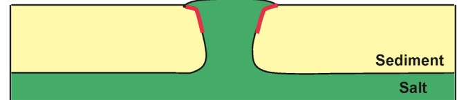
Figure 2. (A) Relationship between the salt/sediment boundary angle ( \alpha ), and the ratio of gross salt flow rate ( R_{sg} ) and the rate of aggradation ( R_a ). (B) Schematic figure showing the three main configurations of salt/sediment boundaries based on the R_{sg}/R_a ratio (based on Talbot, 1995).
