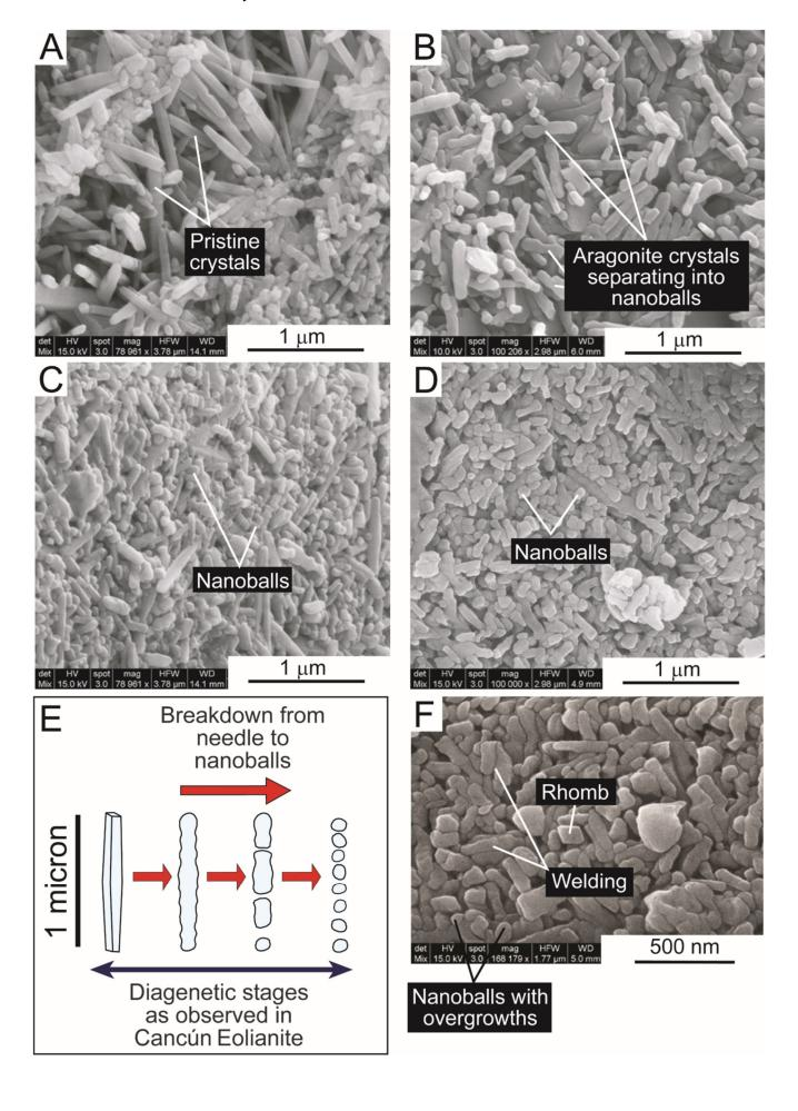
(FACING PAGE) Figure 10. Diagenesis of aragonite crystals. (A) Layer of pristine aragonite crystals. Other layers contain nanoballs. (B) Initial separation of aragonite crystals into nanoballs. (C) Abundant nanoballs and irregular aragonite crystals. (D) Predominance of nanoballs. (E) Stages of aragonite crystal transformation. (F) Possible calcite initiation and welding of crystals.
