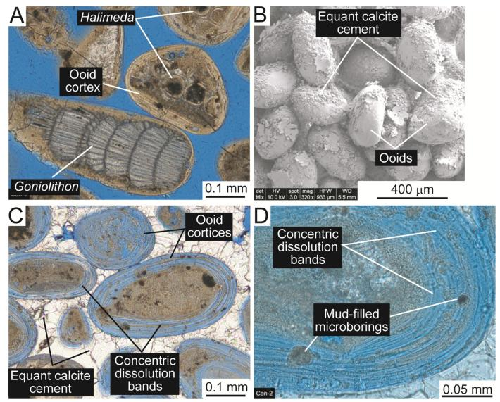
Figure 3. Examples of Cancún ooids. (A) Thin section of unaltered ooids. *Halimeda* and *Goniolithon* are the nuclei. (B) SEM images of ooids with a light coating of equant calcite cement. (C) Thin section showing ooids with thick cortices and well-developed dissolution bands. (D) Close-up of thin-section photomicrograph of concentric dissolution bands.
