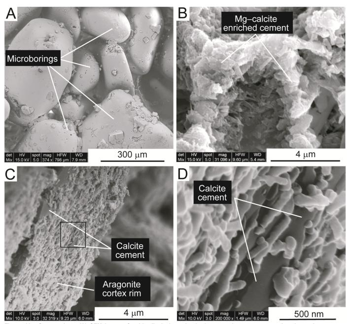
Figure 11. Cementation. (A) SEM image of ooids displaying microborings, meniscus cement, and grain-coating cement. (B) Mg-enriched aphanitic calcite cement precipitated around microboring. Mg enrichment was determined by EDS analysis on the FESEM. (C) Micron-sized calcite crystals embedded in aragonite crystals within ooid band. (D) Close-up of C showing the calcite crystal growing around and incorporating aragonite needles and nanoballs.
