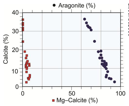
Figure 9. Scattergram based on XRD analysis showing the decrease in aragonite and Mg-calcite as calcite increases. This is evidence that the dissolution of aragonite and Mg-calcite supplies calcium carbonate to form calcite vadose cements. Note that aragonite is dissolving faster than Mg-calcite.
