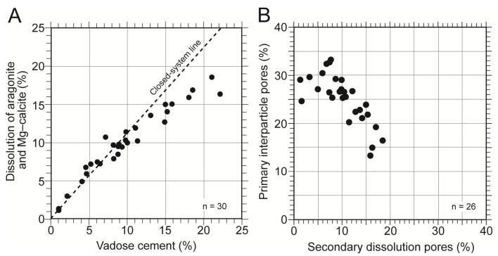
Figure 16. Mass-balance relationships. (A) Scattergram based on thin-section point-count analysis showing relationship between vadose cement and dissolution of aragonite and Mg-calcite. Dashed line shows ideal relationship between aragonite and Mg-calcite with 15% micropores (assumed average percent of micropores based on SEM analysis) versus calcite reprecipitation in a closed system. (B) Scattergram of the covariance of primary interparticle porosity and secondary dissolution porosity.
