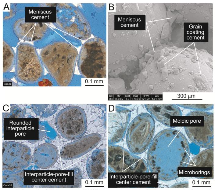
Figure 13. Cementation. (A) Meniscus cement. (B) SEM image of meniscus cement and grain-coating cement. (C) Interparticle pore-fill center cement. Ooid cortices have well-developed concentric dissolution bands. (D) Interparticle pore-fill center cement. Ooid cortices have well-developed concentric dissolution bands. Ooid grain in center has moldic pore outlined by mudfilled microborings. The dark mud in the microborings may be organic rich.
