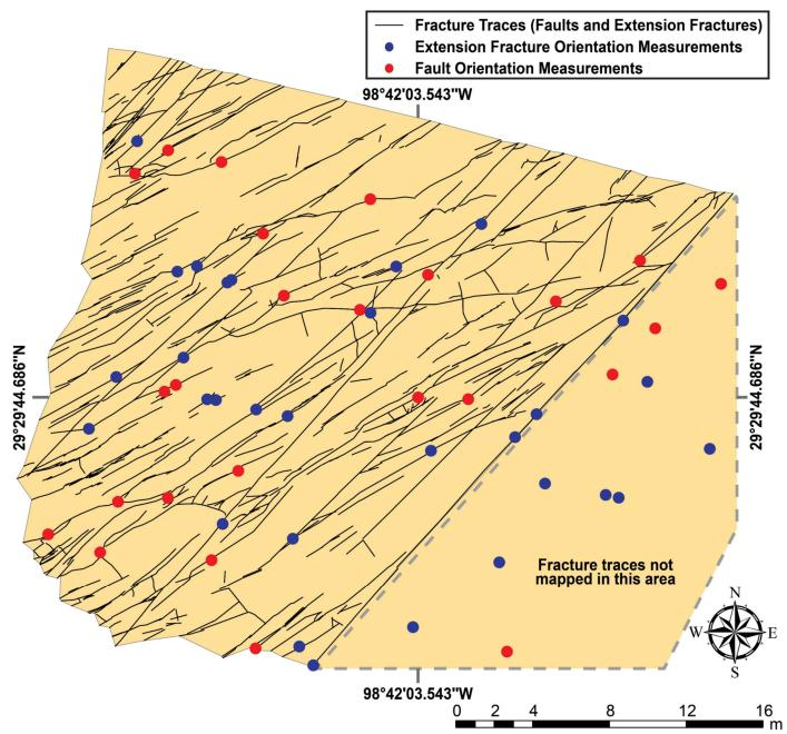
Figure 7. Fracture pavement map from Helotes Creek immediately upstream from the confluence with Culebra Creek with surveyed fracture traces shown as black lines within shaded region, extension fracture measuring locations indicated blue dots, and fault measurement locations indicated by red dots (location AC-3).
