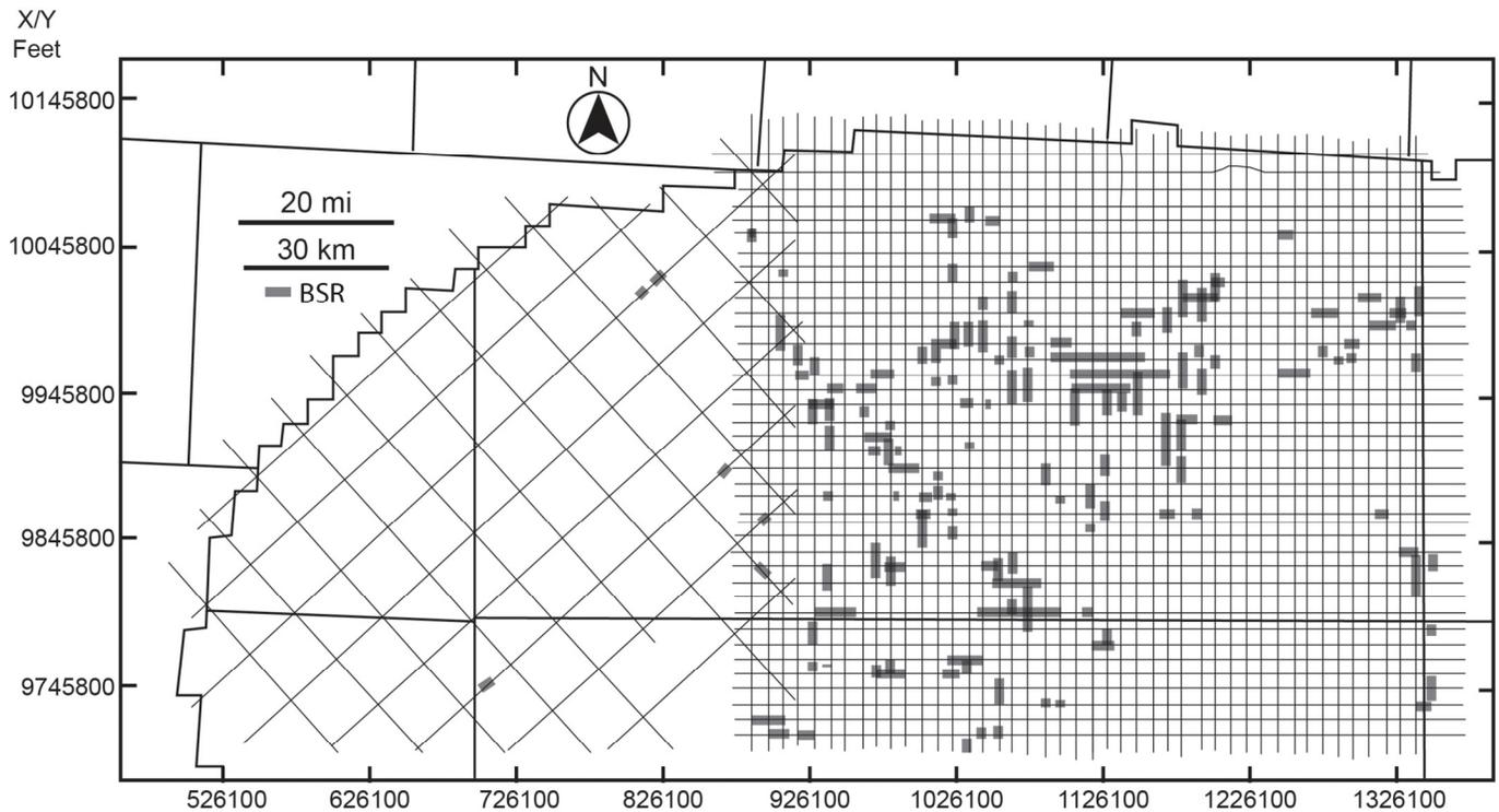
**Figure 9. Locations of interpreted BSRs in the study area. Heavy lines show locations where possible BSRs were observed in the seismic sections.**
