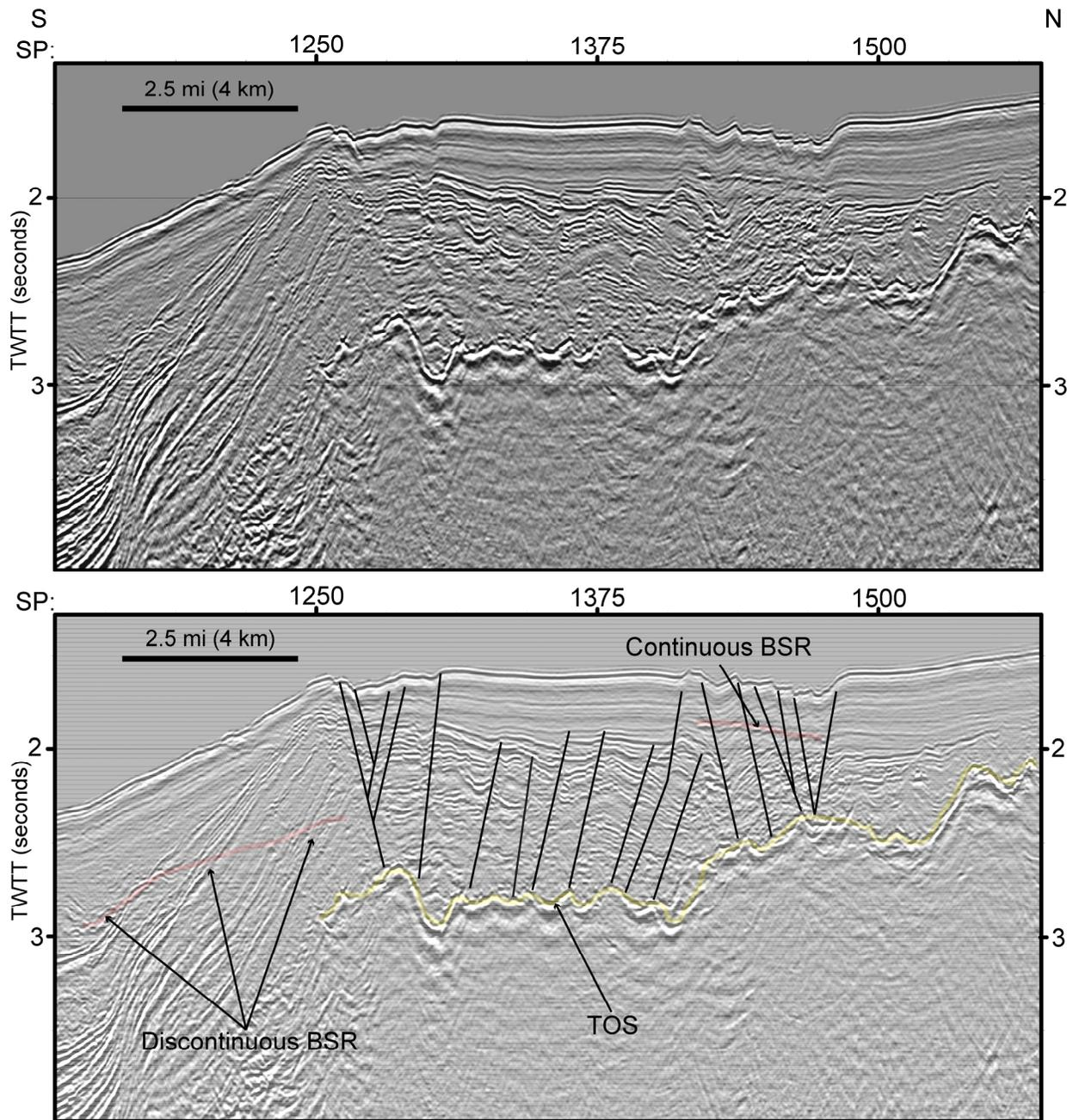
**Figure 7.** Seismic section showing supra-salt faults characteristic of areas in the eastern part of the survey characterized by the presence of salt canopies and sheets. Two examples of BSR are shown in the plot, one continuous and the other discontinuous. Vertical scale is in seconds TWTT, and horizontal scale lists shotpoint numbers. Vertical exaggeration is 10:1. Location of section is shown in [Figure 2](#).
