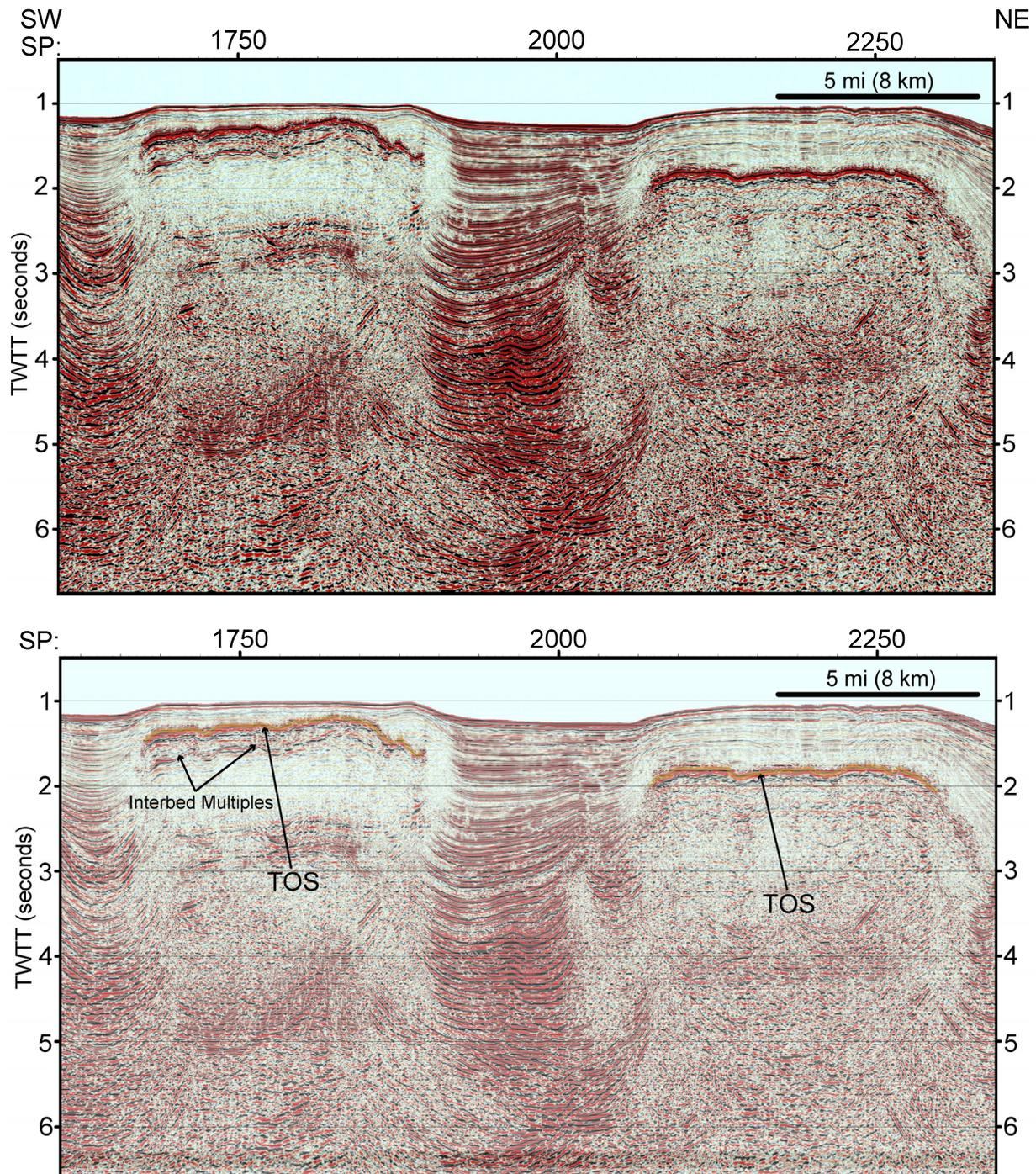
Figure 5. Seismic section showing isolated salt diapirs in the western part of the study area. TOS is indicated by arrows. Vertical scale is in seconds TWTT and horizontal scale lists shotpoint numbers. Vertical exaggeration is 4:1. Location of section is shown in Figure 2.
