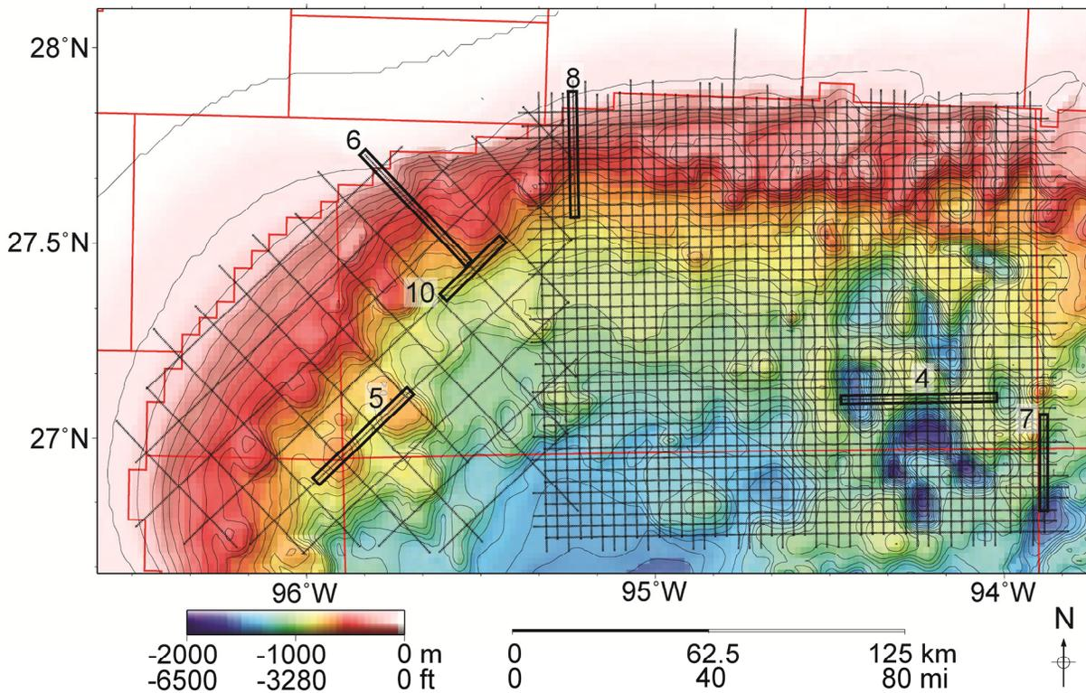
Figure 2. Bathymetric map of the study area with seismic lines superimposed. Numbered line segments are shown in subsequent figures, with numbers denoting figure numbers. Bathymetry contours are shown in 100 m (~330 ft) intervals (bathymetry from Smith and Sandwell, 1997).
