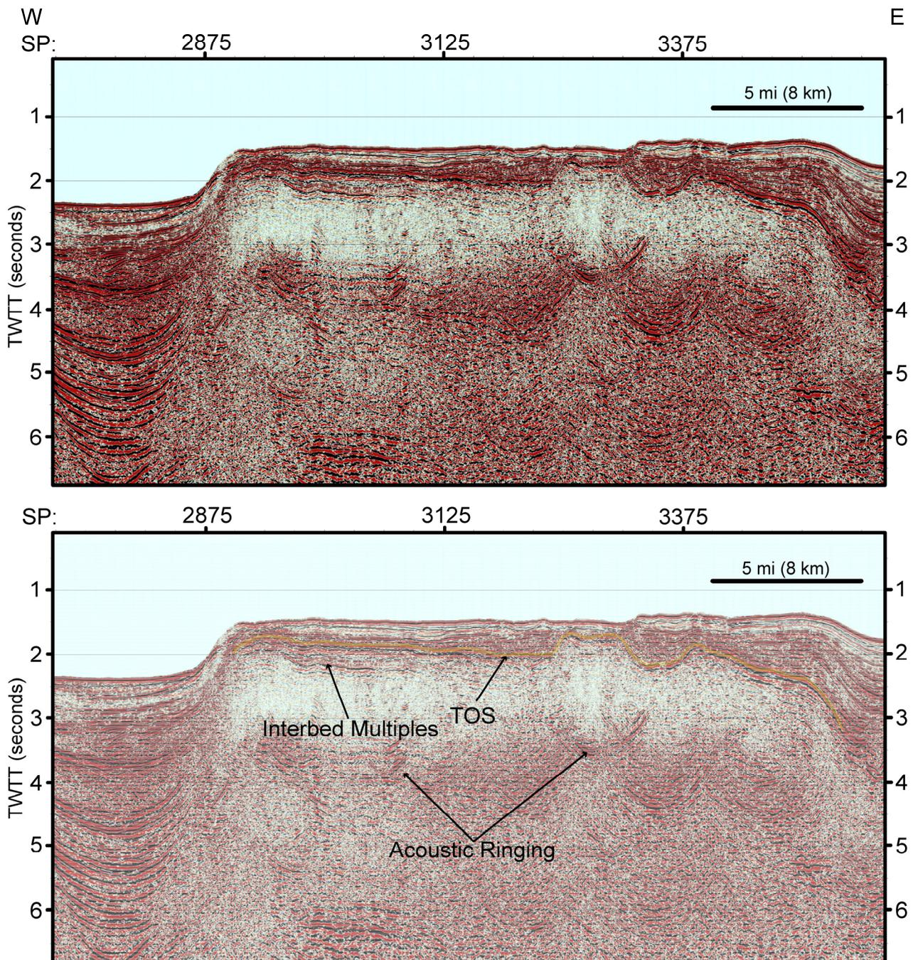
**Figure 4.** Seismic section showing salt sheet body in the southeast part of the survey area. Examples of interbed multiples are shown as well as acoustic ringing. Vertical scale is in seconds TWTT, and horizontal scale lists shotpoint numbers. Vertical exaggeration is 4:1. Location of section is shown in [Figure 2](#).
