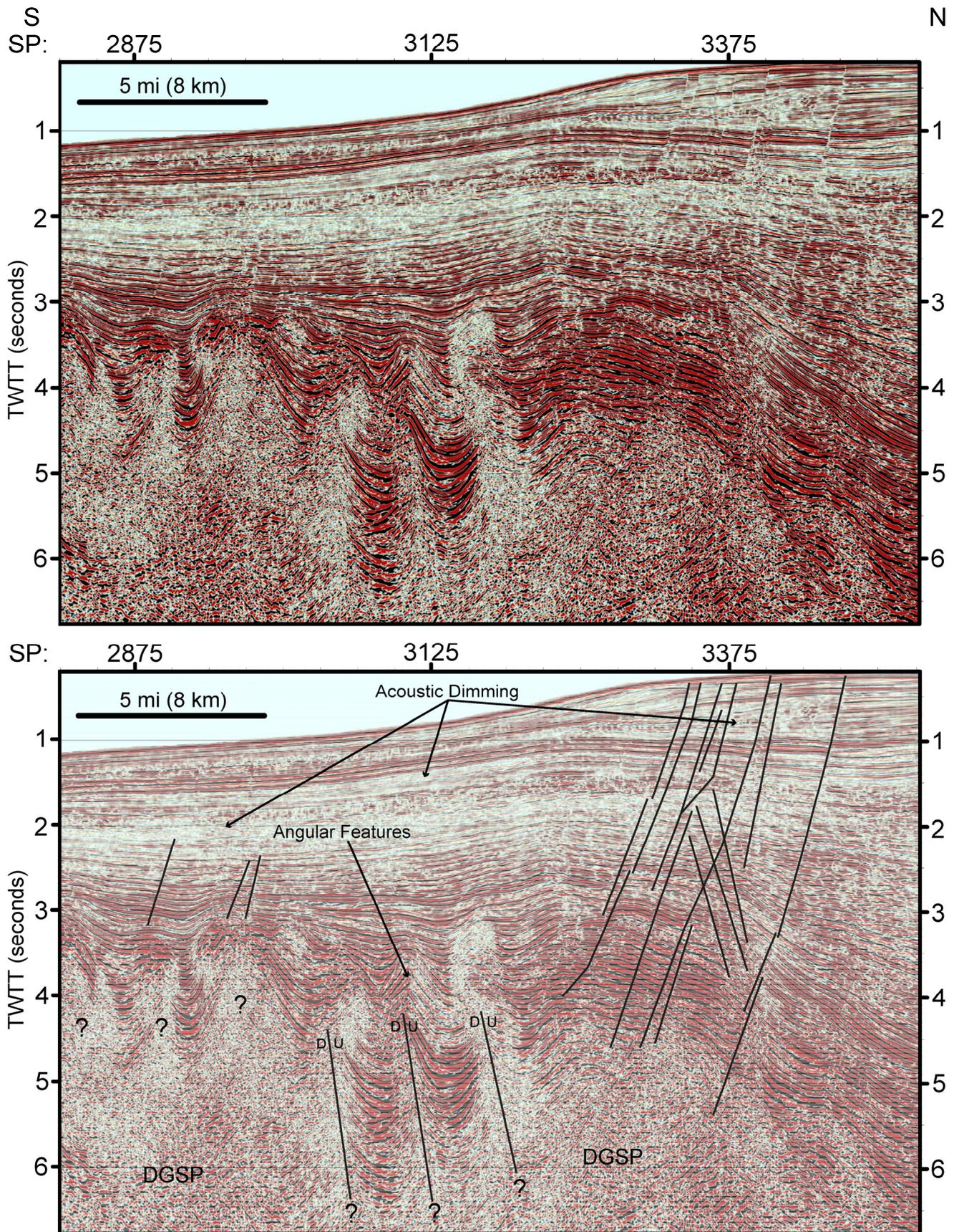
Figure 8. Seismic section showing DGSP. This section of the DGSP has some resolvable bedding that we have interpreted as thrust faults (lower center). U/D symbols indicates upthrown and downthrown blocks, respectively. Some angular bedding is observed. Acoustic dimming (gas indicator) areas are indicated by arrows. Vertical scale is in seconds TWTT, and horizontal scale lists shotpoint numbers. Vertical exaggeration is 4:1. Location of section is shown in [Figure 2](#).
