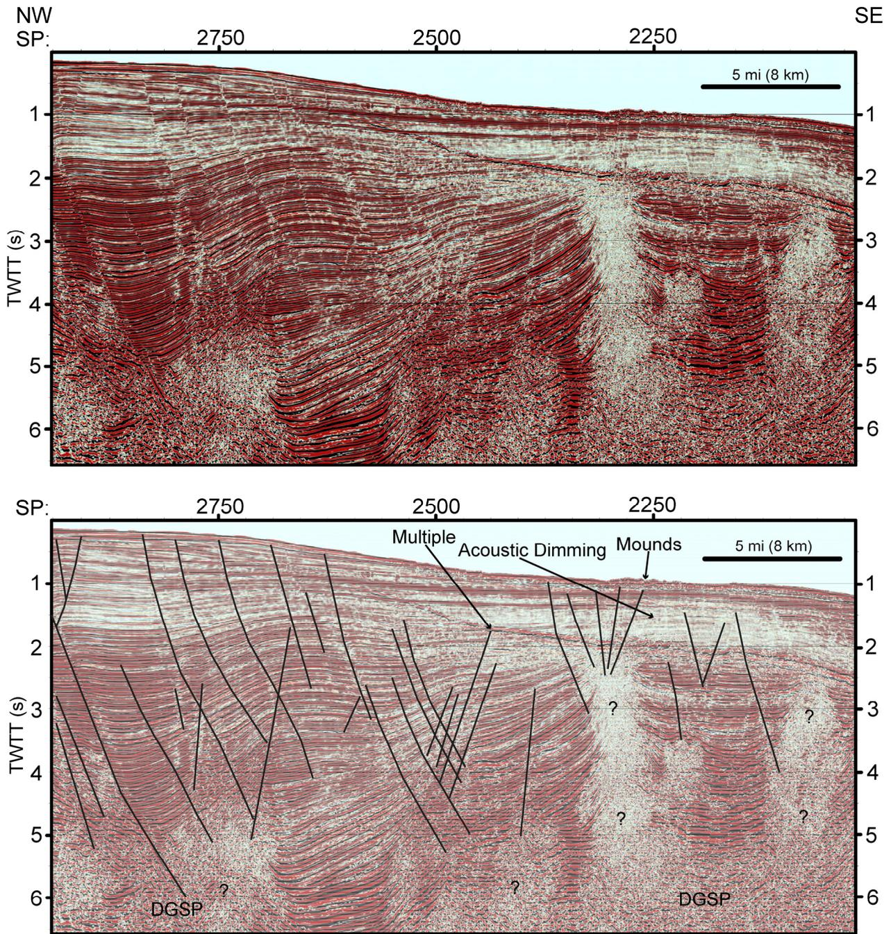
Figure 6. Seismic section showing regional faults produced by gravitational sliding (both regional and counter-regional faults are observed in the plot), vertical gas features (part of DGSP), and acoustic dimming zone. Mounds, a multiple, and acoustic dimming are indicated by arrows. Vertical scale is in seconds TWTT, and horizontal scale lists shotpoint numbers. Vertical exaggeration is 4:1. Location of section is shown in Figure 2.
