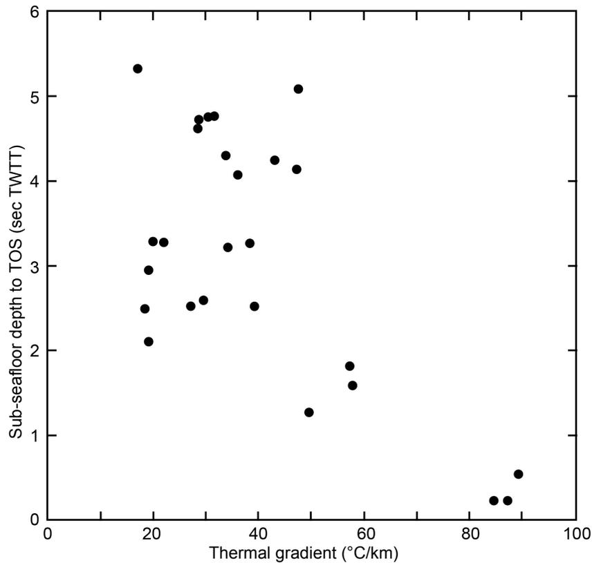
**Figure 11. Thermal gradient values measured in the study area plotted versus sub-seafloor depth to the top of salt (in seconds TWTT).**
