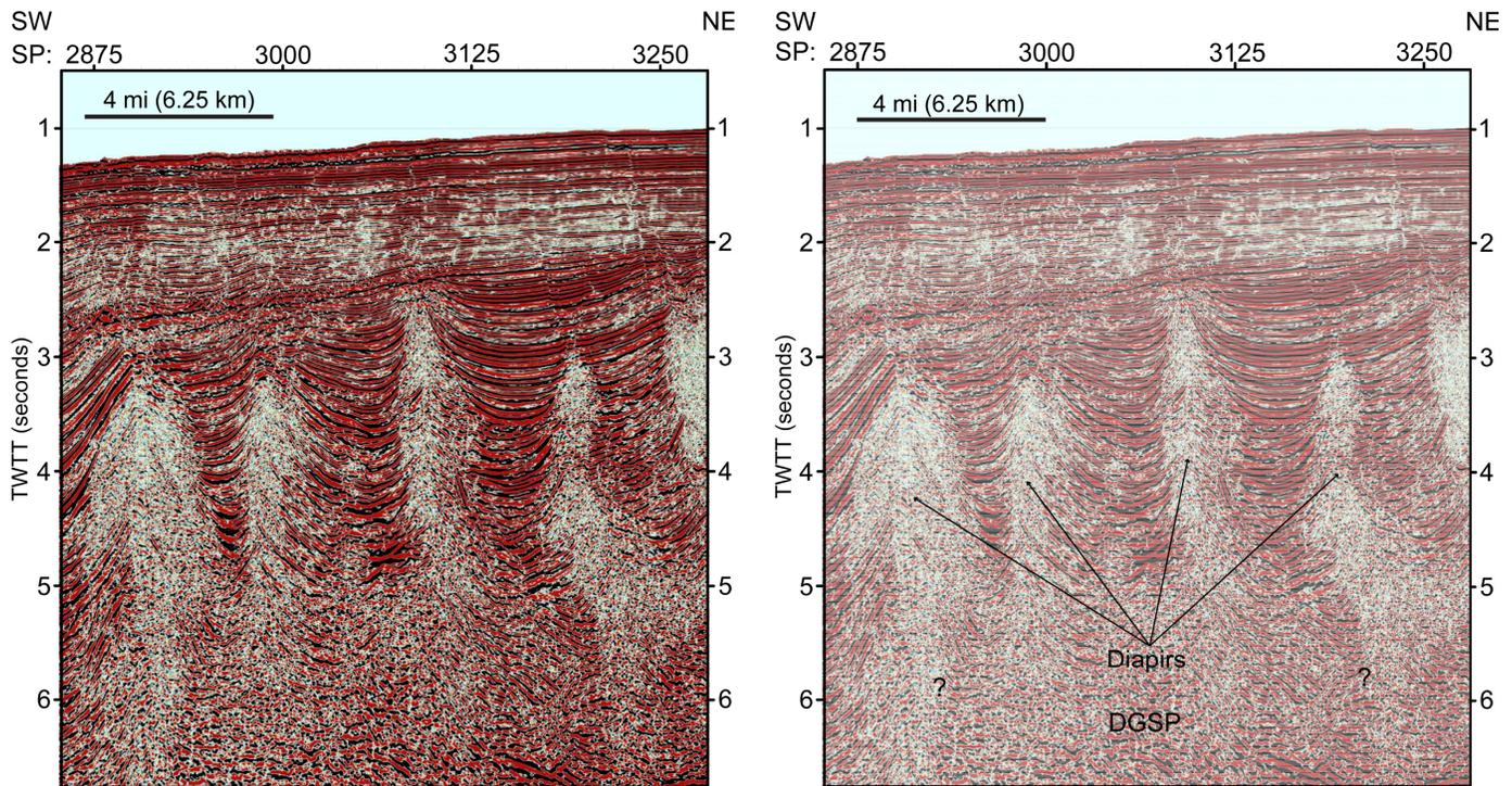
**Figure 10. Seismic section showing the DGSP. This section of the DGSP shows the diapir-like structures. Vertical scale is in seconds TWTT, and horizontal scale lists shotpoint numbers. Vertical exaggeration is 4:1. Location of section is shown in Figure 2.**
