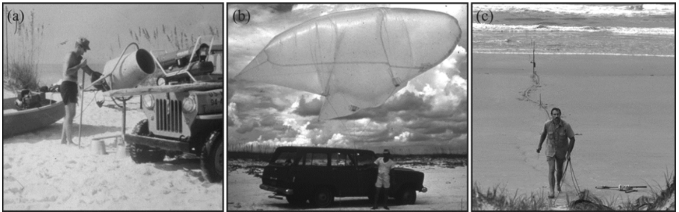
Figure 5. (a) Norwood Rector of the CSI Field Support Group dying sand for an early 1970s sediment tracer experiment along the beach at Ft. Walton, Florida. (b) A tethered balloon used to carry a camera package for photographing rhodamine dye as water circulated through rhythmic beach and nearshore bar morphology in the early 1970s. (c) Joe Suhayda setting up an experiment to measure waves as part of a coastal processes study along a Brazilian beach in 1976.
