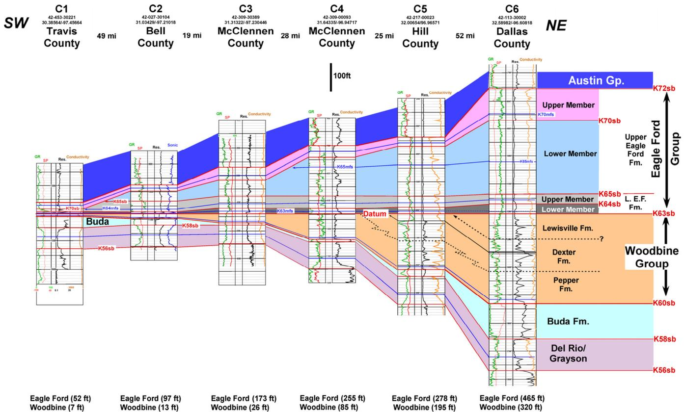
**Figure 17.** Well-log cross section illustrating distribution and thickness variations of the depositional sequences (allostratigraphic) units correlated from Dallas County to Travis County in the shallow subsurface along the western flank of the East Texas Basin. Location of well-log cross section on Figure 1.
