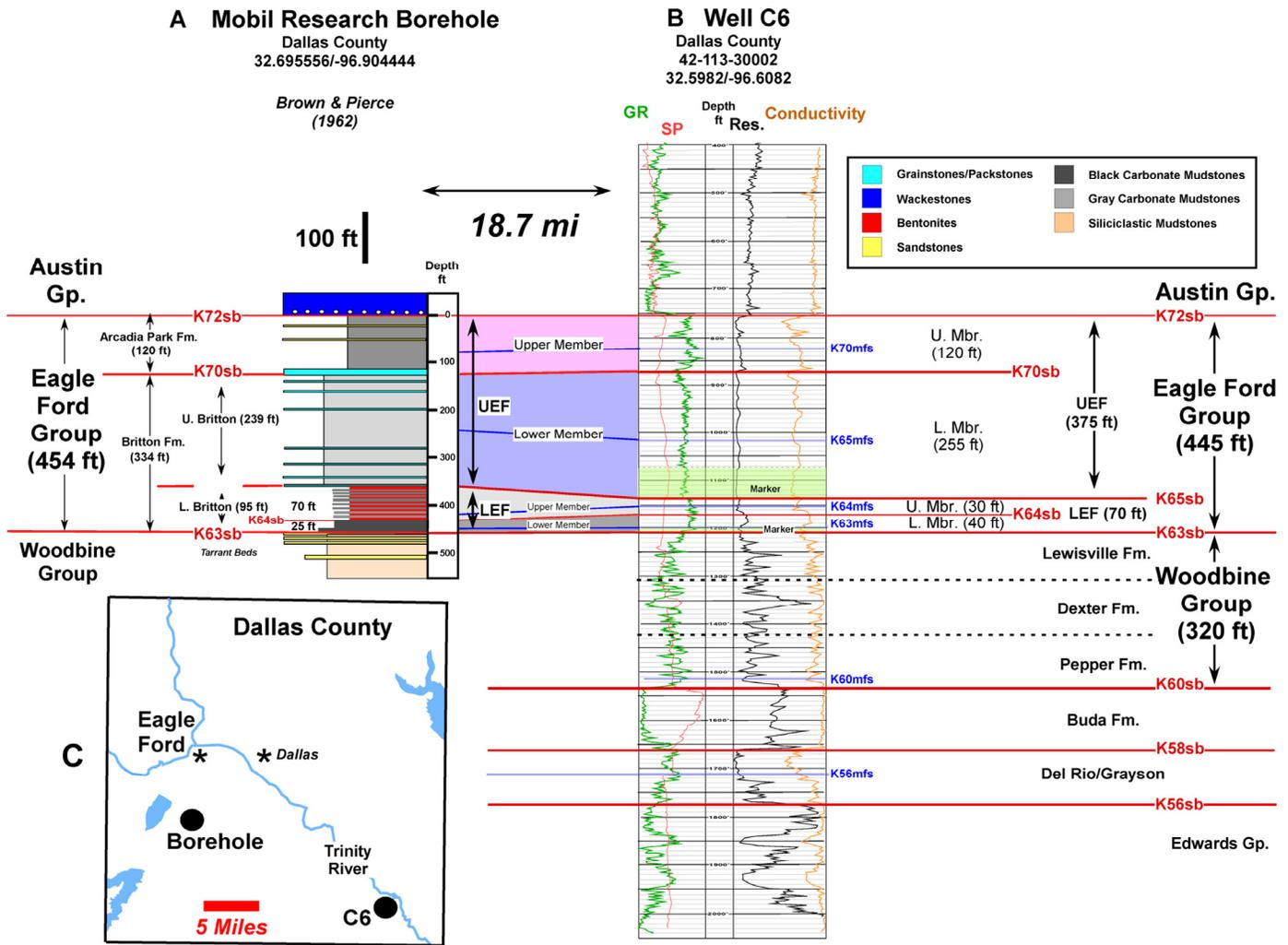
Figure 16. (A) Lithostratigraphic units in the Mobil's Dallas Area Eagle Ford borehole defined by Brown and Pierce (1962) and in this paper. (B) Borehole to well-log tie of the sequence stratigraphic surfaces and units from the Eagle Ford Borehole to Well C6 in Dallas County, Texas. (C) Location map illustrating the location of: (1) Eagle Ford, Texas, (2) the Mobil Research Borehole, and (3) Well C6.
