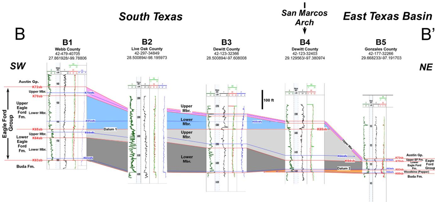
Figure 9. Well-log cross section illustrating distribution and thickness variations of the depositional sequences units correlated from South Texas to the southwest corner of the East Texas Basin. Location of well-log cross section on Figure 1.
