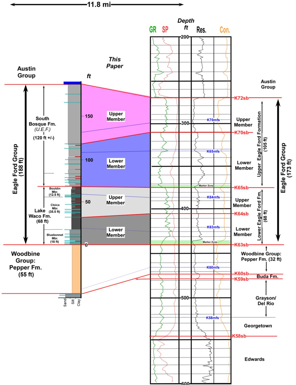
Figure 15. Outcrop to subsurface tie of the sequence stratigraphic surfaces and units from the Cloice Branch area near Waco to Well C3 in McClennen County, Texas. Legend for lithologies is shown on Figure 13.
