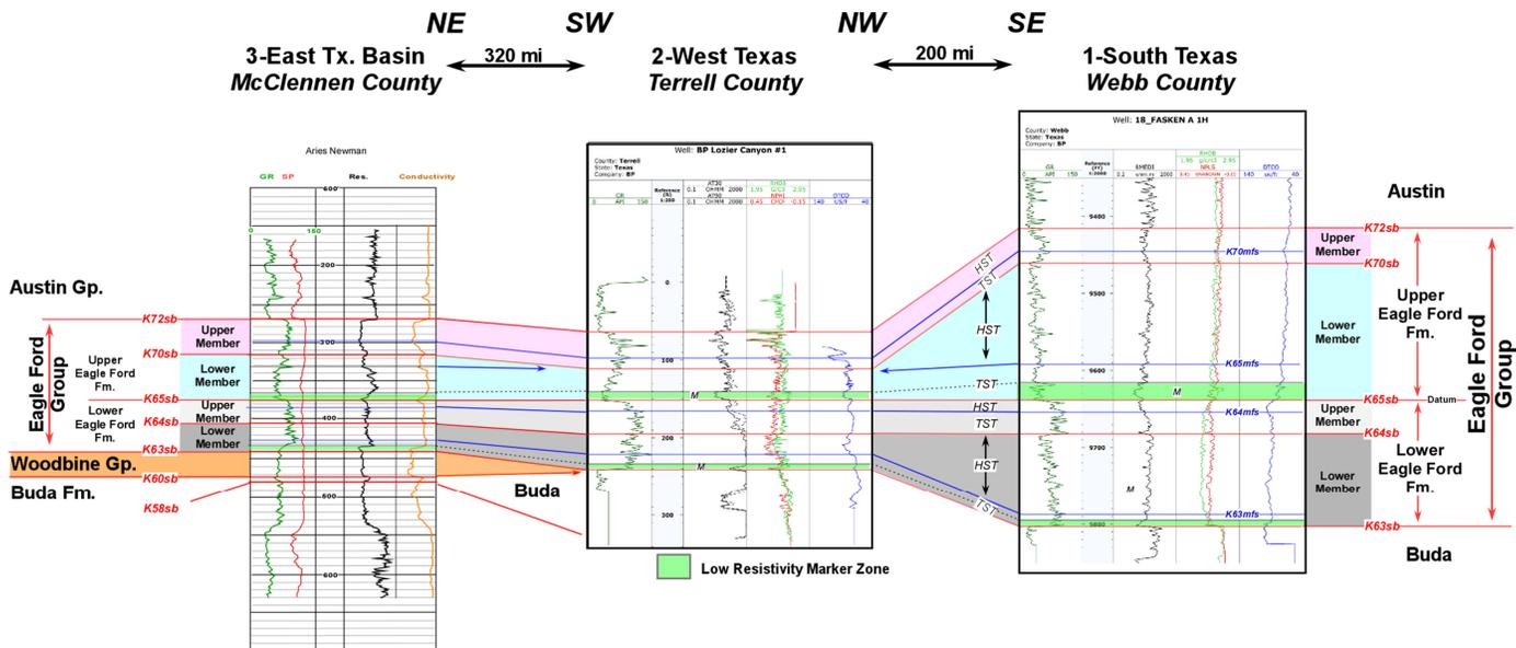
Figure 8. Type well-log cross section of the sequence surfaces and units correlated from West Texas, to South Texas, and into East Texas Basin. Location of wells on Figure 1.
