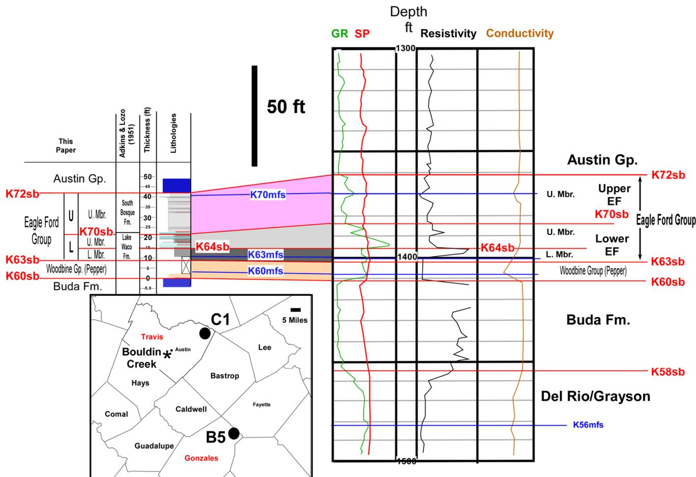
Figure 11. Outcrop to subsurface tie of the sequence stratigraphic surfaces and units from Bouldin Creek to Well C1 in Travis County, Texas.
