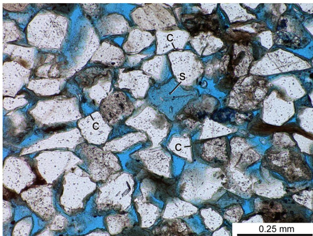
**Figure 6.** Continuous chlorite coats (C) inhibited quartz cementation in upper Wilcox sandstone from the Shell #2 Muzza well, Fandango Field, Zapata County, Texas, at a depth of 15,182 ft (4627.5 m). Sample contains only 1% quartz cement at a temperature of 397°F (203°C). Secondary pore (S) is outlined by chlorite cement. Porosity = 25.6% and permeability = 68 md. Average grain size is 3.16 phi (0.112 mm). Plane-polarized light.
