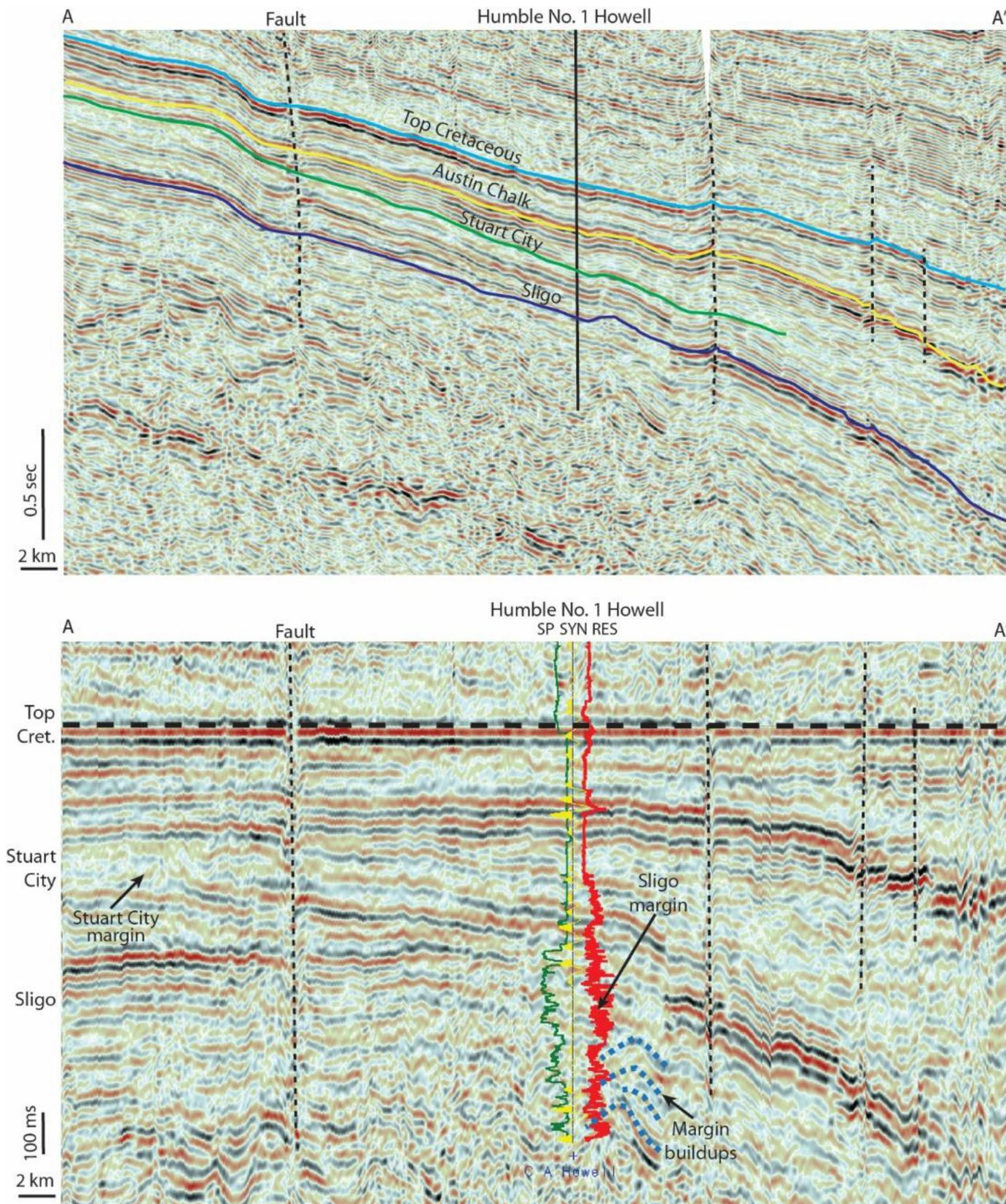
Figure 4. GulfSpan GSM3-2150 2D seismic line showing the location of the core relative to Sligo and Stuart City (Edwards) shelf margins. The top panel (unflattened) shows the architecture of the present-day Cretaceous platform; the bottom panel shows the same interval, flattened on top of the Cretaceous. Major formation boundaries are labeled, and annotations show faults and seismic facies (buildups) of note. Seismic authorized for publication courtesy of Fairfield Geotechnologies.
