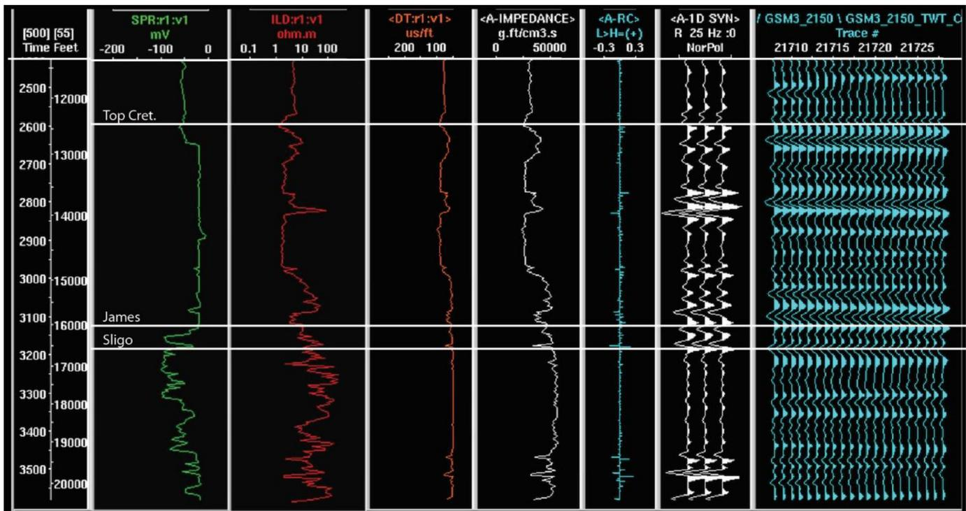
Figure 5. Synthetic seismogram for the Humble No. 1 Howell well projected to seismic line A–A'. The impedance log is calculated from the acoustic (delta time) log and Gardner's equation.
