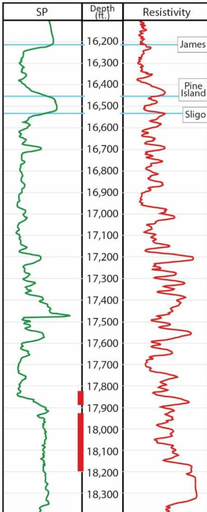
Figure 3. Wireline log for the Humble No. 1 Howell well. James, Pine Island, and Sligo formation tops are delineated by light blue lines and labeled. Cored intervals studied are shown by vertical red bars.
