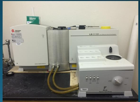
Laser diffraction particle size analyzer
