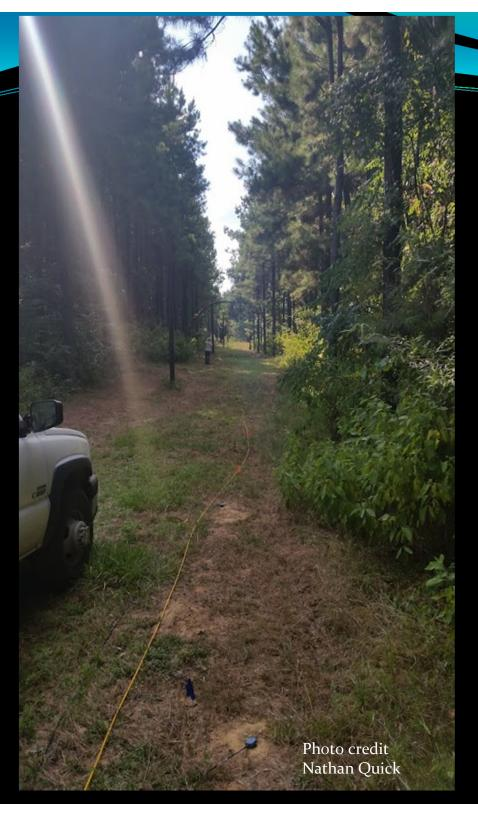
144 receiversone 715 m line5 meter spacing1 ms sample rate4 sec records
