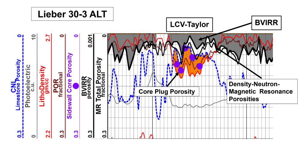
$$Swirr = \frac{BVIRR - Magnetic \ Resonance}{PHI - Density - Neutron}$$
