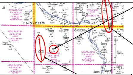
The Turner horizontal well (Linam) did not produce as well in the Turner. The Upper Mcferren completions in the Webb 13-5H here produced 50% more than the Linam 23-1H placed in the Turner
