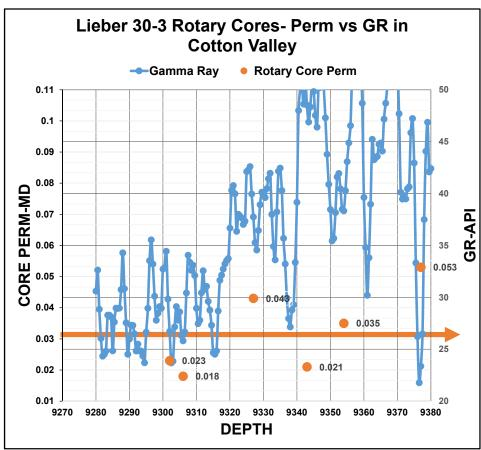
As GR increases Porosity increases in this clay contaminated interval
