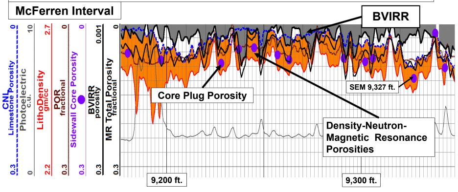
$$Swirr = \frac{BVIRR - Magnetic Resonance}{PHI - Density - Neutron}$$
