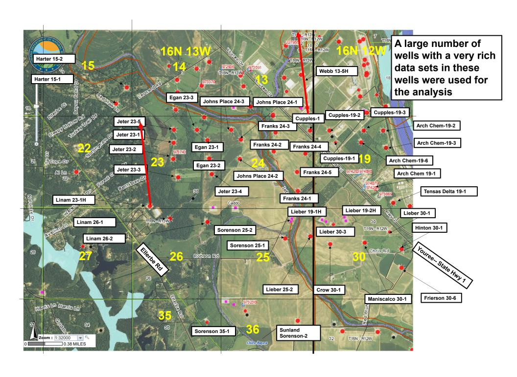
The Aethon Webb 13-5H ALT is higher in the ssection and produced 3-Bcf from a 3250ft lateral → 1-Bcf/1000ft using 2008 technology
