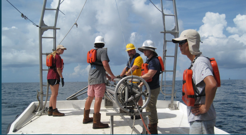
Submersible vibracorer used for this study to collect cores up to 5 meters in length. Image by: Kristine DeLong
